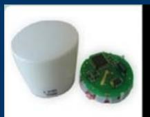
The MEMS monitor is composed of a microswitch, a clock and a memory.
